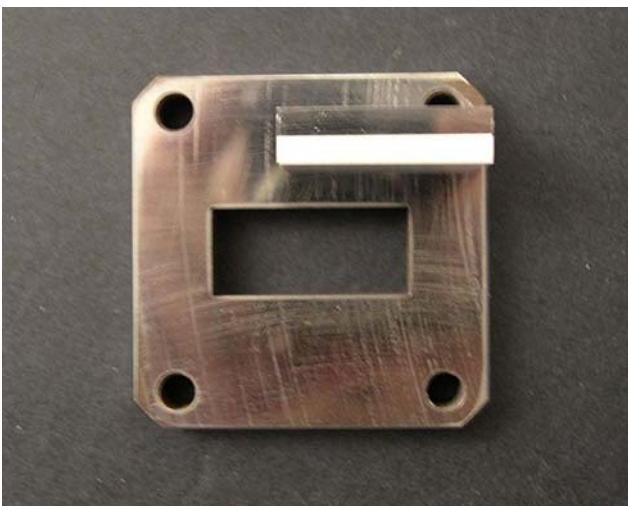
Fig. 9 Metal backed samples for WR-90 X-band holder. Sample size = 22.86 \times 10.16 \times 6.00 mm; coating thickness = 3^{\pm 0.1} mm; substrate thickness = 3^{\pm 0.1} mm
